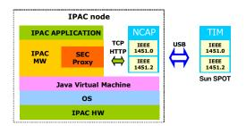
Figure 2. An IEEE 1451-compliant architecture based on Sun SPOTs.
