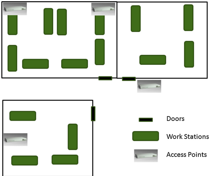
Fig. 9 Physical topology. Offices layout and AP placement
