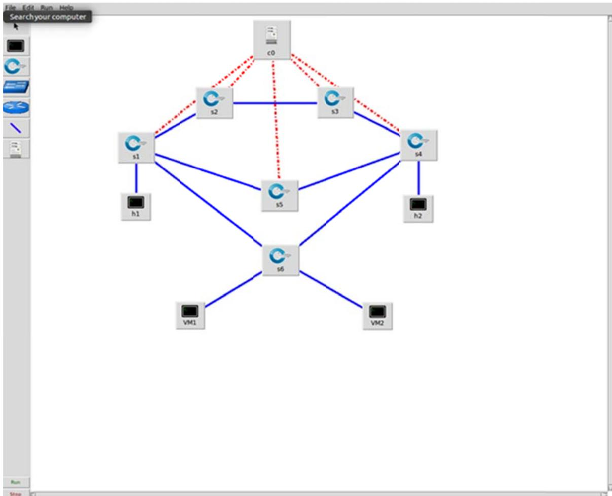
**Figure 4: Network in a box proposed topology**
