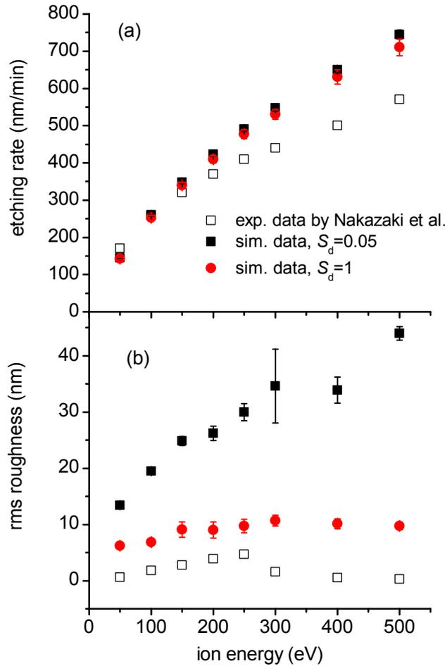
**Figure 3:** a) The etching rate and b) the rms roughness vs the ion energy as obtained from our simulation and the measurements of Nakazaki et al. [20]. The simulation results refer to cases 0014 to 0029: Two values of  $S_d$  are considered:  $S_d=0.05$  and  $S_d=1$ . The error bars are coming from the standard deviations of the runs of each case
