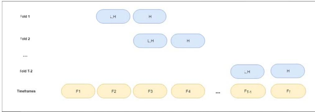
**Figure 6: Test Sets using Time Series Cross Validation**
