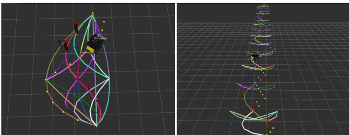
**Figure 1: Candidates and selected path (dotted) for a 45° slope (left) and a longer 43° slope (right).**
