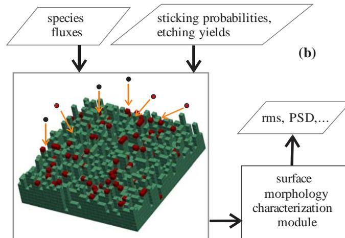
**Figure 2: Schematic with the inputs and the outputs of the MC modeling framework**
