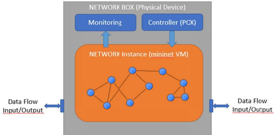
**Figure 2: The SDN-based Network BOX**
