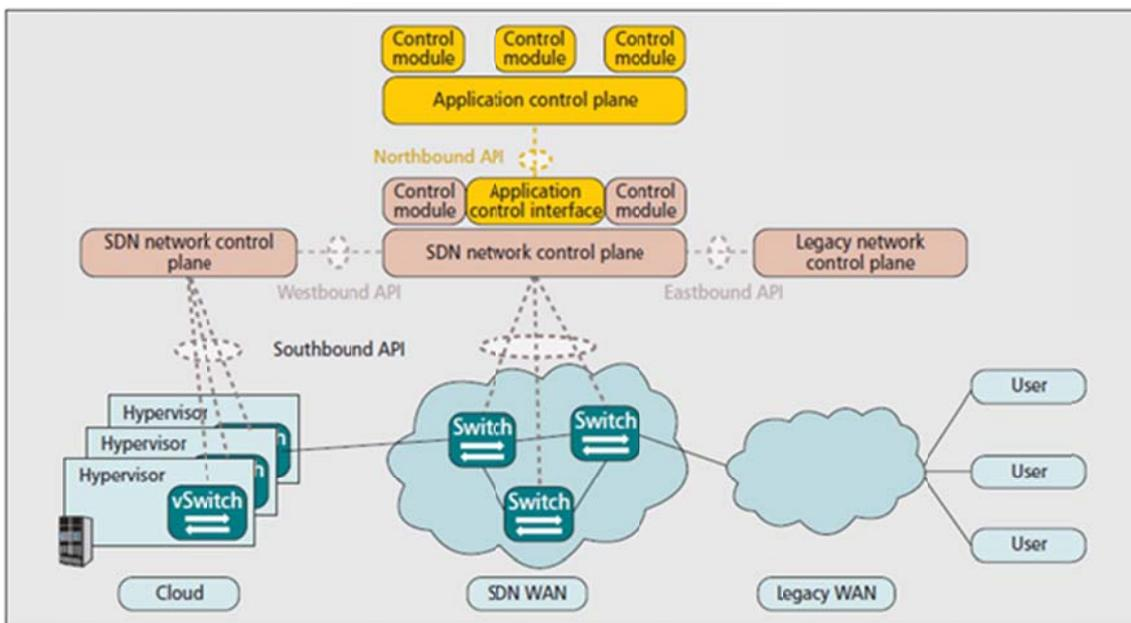
Figure 1: The high-level SDN architecture
