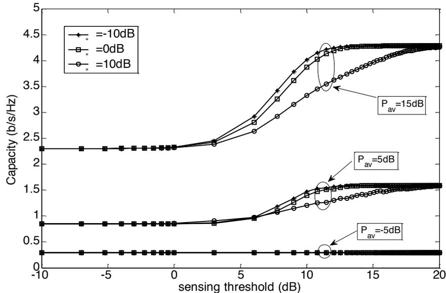
**Fig. 3** Capacity  $C_s$  vs. sensing threshold  $\eta$  for different  $\gamma$  and  $P_{av}$  assuming  $I_{pk} = 0dB$
