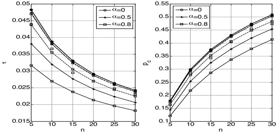
**Fig. 6.** Transmission probability  $\tau$  (left part) and collision probability  $p_c$  (right part) vs. number of stations  $n$  for different activities  $a$  with  $C = 1$  channels (solid lines), with  $C = 3$  channels (dashed lines) and with  $C = 6$  channels (dotted dashed lines).
