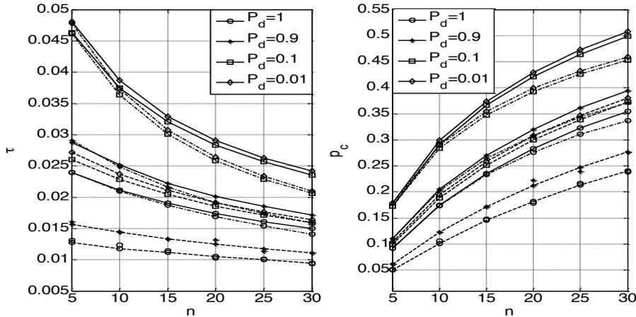
**Fig. 5.** Transmission probability  $\tau$  (left part) and collision probability  $p_c$  (right part) vs. number of stations  $n$  for different probabilities of detection  $P_d$  with backoff stage  $m = 3$  and contention window  $W = 32$  (solid lines), with  $m = 3$  and  $W = 64$  (dashed lines) and with  $m = 5$  and  $W = 32$  (dotted dashed lines).
