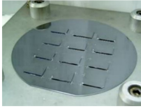
Fig. 2. Four-inch Si wafer with multiple dies bonded on specific regions
