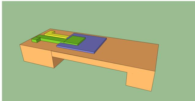
**Figure 5:** Illustrated schematic of the cantilever-based MEMS microgenerator
