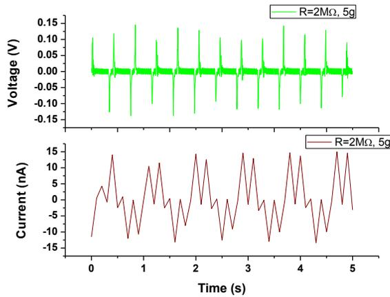
**Graph 12:** Voltage and Current output of an Al nanogenerator over a  $R_L=2M\Omega$  for given acceleration.
