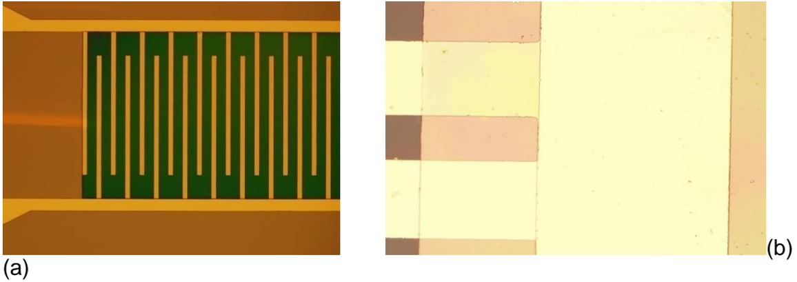
Figure 4: (a) Intedigitated electrodes, (b) Top-Bottom electrodes.
