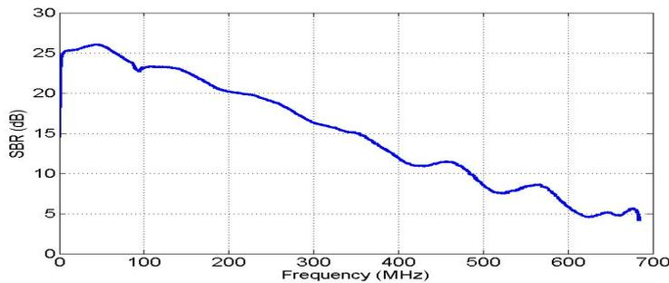
**Fig. 13:** Measured SNR per subchannel
