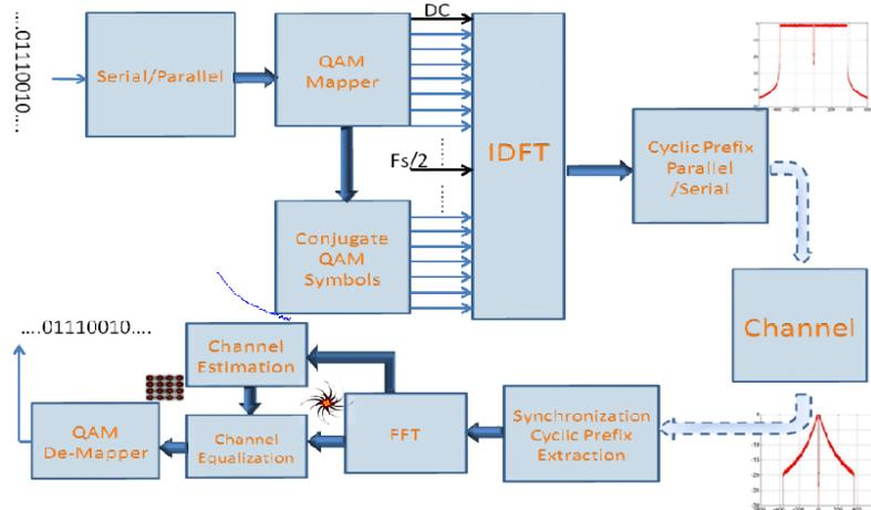
**Fig. 3:** Block diagram of the DMT transceiver
