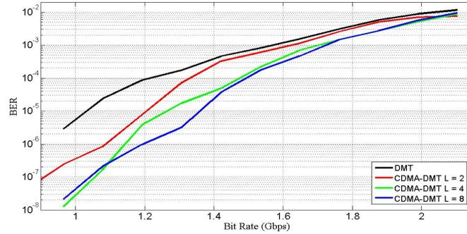
**Fig. 11:** Comparative results of BER versus net transmission rate for CDMA-DMT and DMT for the case of 32-QAM and 50m SI-POF
