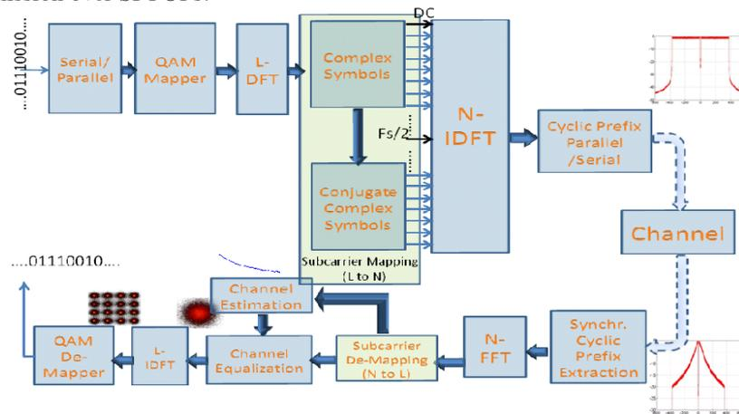
**Fig. 4:** Block diagram of the DFT Spread DMT transceiver
