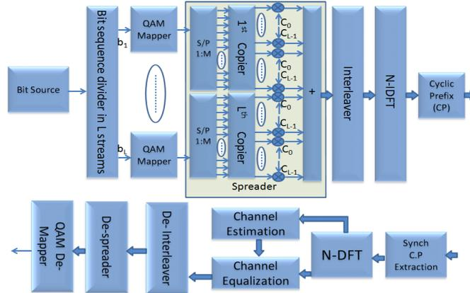
**Fig. 5:** Block diagram of CDMA-DMT transmitter and receiver
