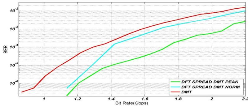
**Fig. 8:** Comparative results of BER versus net transmission rate for DFT-spread DMT and DMT for the case of 64-QAM and 50m SI-POF
