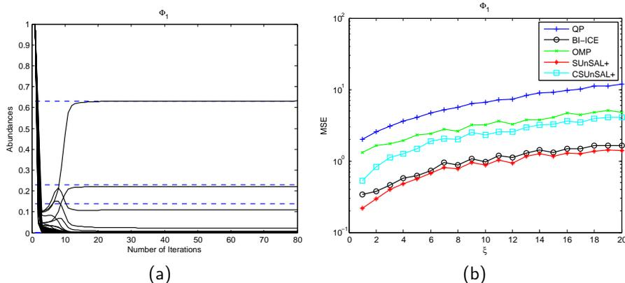
**Fig. 1.** (a) Estimation of the entries of the sparse vector  $\mathbf{w}$ , as BI-ICE progresses. The algorithm is applied to simulated data, generated using a highly correlated matrix of spectral data. White noise is added (SNR = 25 dB). Dashed lines: true values. Solid lines: estimated values. (b) MSE as a function of the level of sparsity obtained by different unmixing methods when applied to simulated data with white additive noise (SNR = 20 dB)
