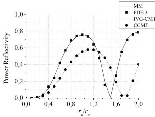
**Fig 3.** Comparison of power reflectivity calculated by MM, FDFD, IVG-CMT and CCMT for a single defect rod radius  $r_d$  inside a PCW.
