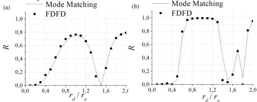
**Fig 1.** Comparison of power reflection coefficient of the MM and the finite difference frequency domain (FDFD) methods for a) single, and b) triple defect rods inside a PCW.
