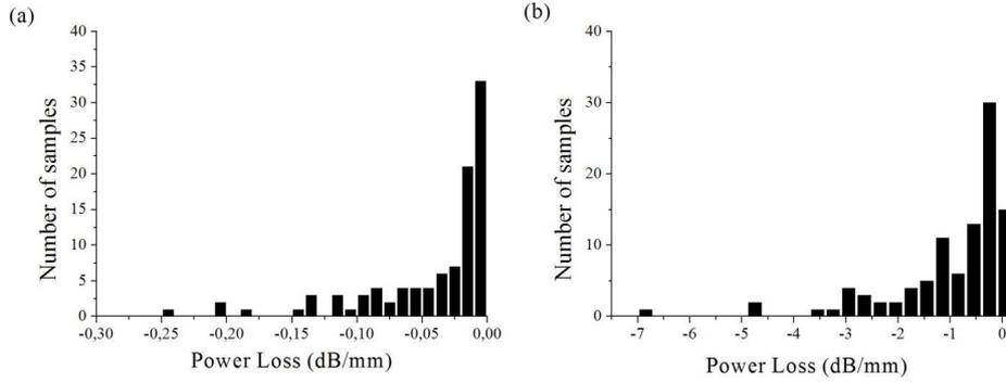
**Fig 2.** Power loss (expressed in dB/mm) due to scattering obtained considering 100 perturbed PCWs assuming a)  $\Delta=1\text{nm}$  and b)  $5\text{nm}$ .
