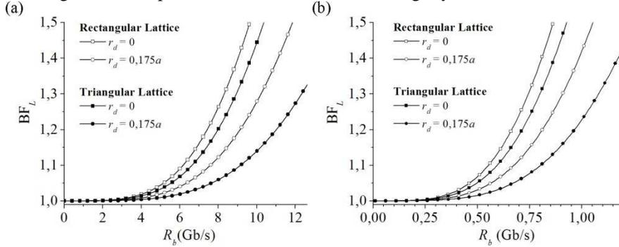
**Fig 7.** Linear Broadening factor for hollow and defect-type PCW waveguide formed in either rectangular or triangular PC lattice at the left band edge when a)  $T_d=1$ ns and b)  $T_d=5$ ns.
