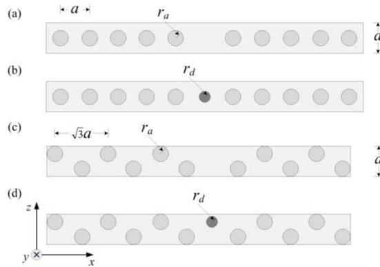
**Fig 5.** Examples of photonic crystal waveguides unit cells formed by a) removing a single rod from a square photonic lattice, b) inserting defect rods in a square lattice, c) removing a rod from a triangular lattice, d) inserting defect rods in a triangular lattice.
