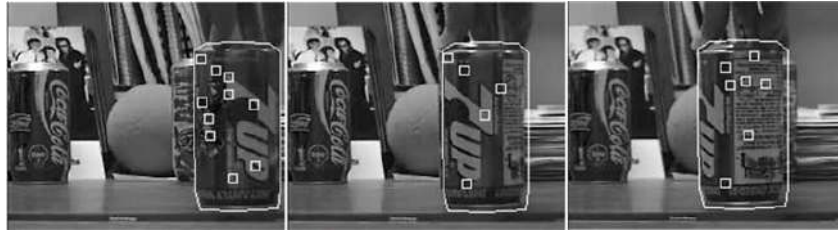
Fig. 6. Tracking Results - 7up Sequence:aHMT, 60 particles, frames 1,180,300
