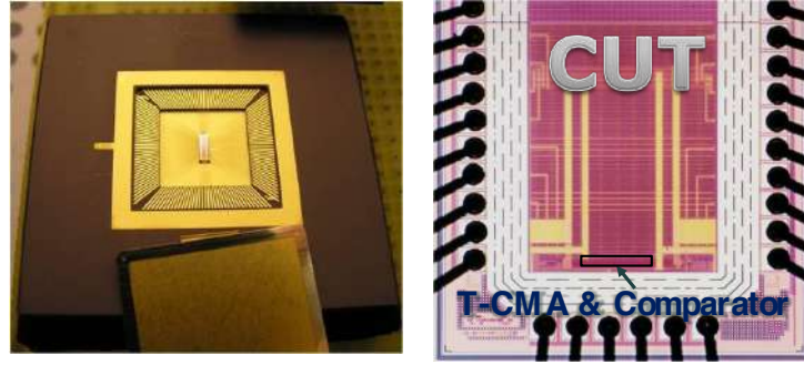
Fig. 12. Fabricated I_{DDQ} test chip and a microphotograph
