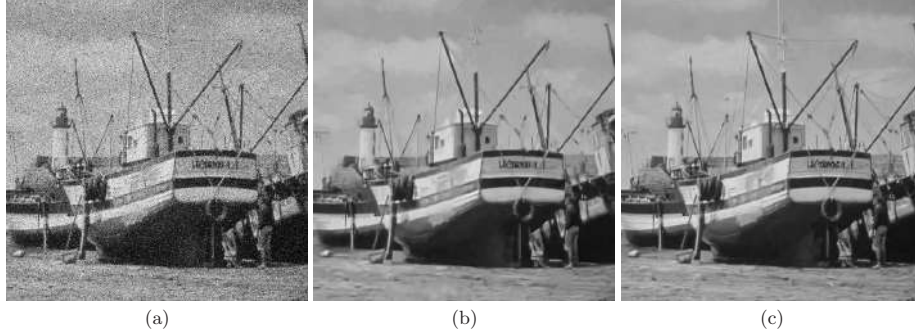
Fig. 6: (a) The boat image corrupted by 20 dB of Gaussian noise and 10% outliers. (b) Denoising with BM3D (28.97 dB). (c) Denoising with joint KGARD-BM3D (31.52 dB).
